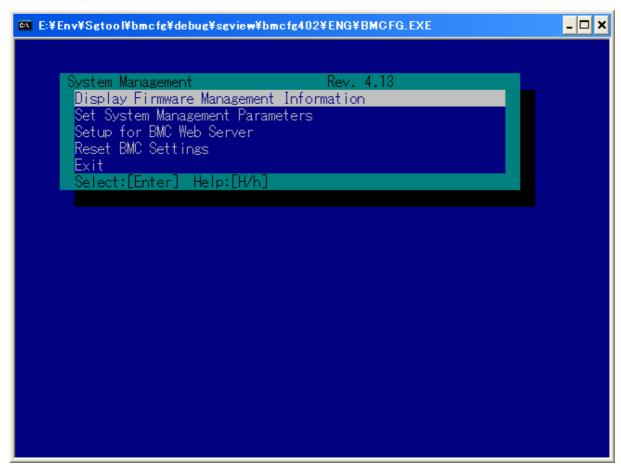
Start the NEC EXPRESSBUILDER CD-ROM in the host system, and select [Tool]-[System Management]-[Setup for BMC Web Server].
