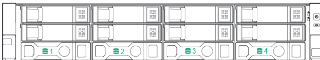
8x 3.5-inch drive model (SAS/SATA HDD)+ 2x2.5 (SAS/SATA HDD/SSD, PCIeSSD)
