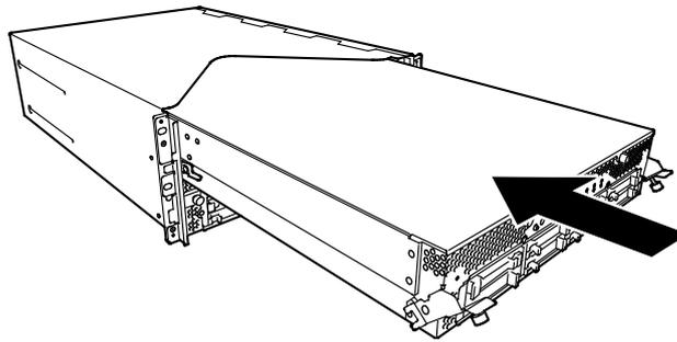
2. Push up the black levers placed on the left and right sides of the front of the CPU/IO module, and fasten them with screws.
