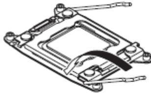
14. Close the socket lever marked with "🔓 ① →" to fix it.
