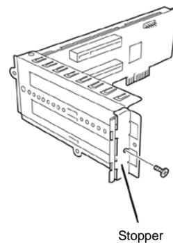
8. Remove the PCI bracket cover.
