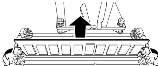
9. Attach the dummy memory module.
