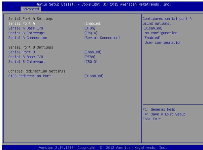
From **BIOS Redirection Port**, select **Serial Port A** or **Serial Port B** and then press **Enter** to display the menu screen shown below.
