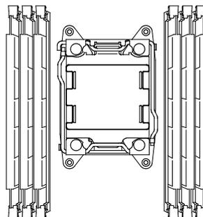
8. Push down the socket lever marked with "↪ ① →" once to unlatch it from the hook, then slowly open the lever until it stops.
