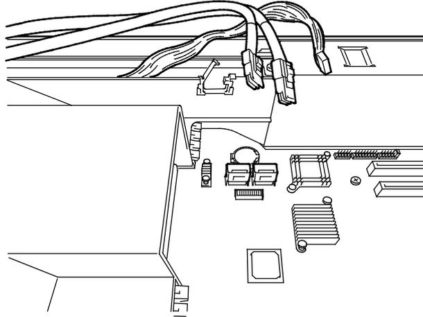
7. Remove the air duct.
