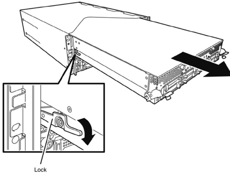
7. Pull out the CPU/IO module gently and carefully, and place it on a flat and sturdy table. Avoid the dusty or humid place.
