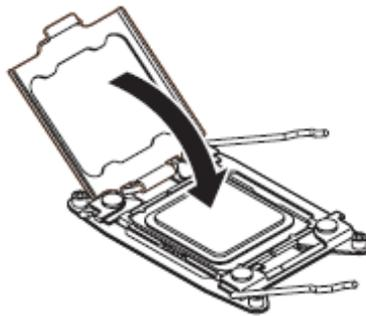
13. Close the socket lever marked with "← 🔒 ①" to fix it.
