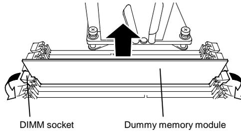
**Important** Keep and store the removed dummy memory module with care.
