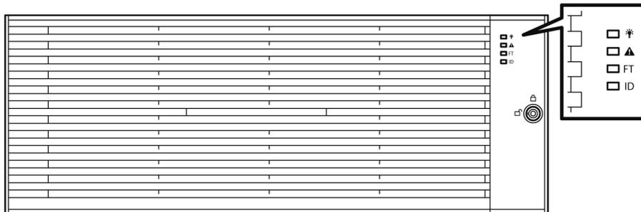
LEDs on hard disk drives installed in 2.5-inch hard disk drive bay
