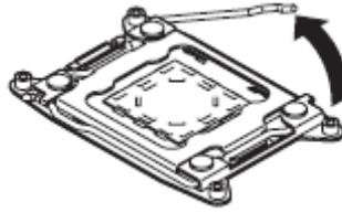
9. Push down the socket lever marked with "← ①" once to unlatch it from the hook, then slowly open the lever until it stops.
