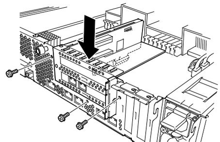
12. Install the stopper and secure it with one screw.
