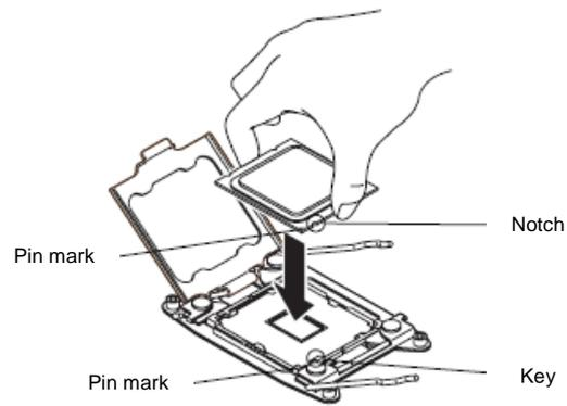
12. Lightly push the processor to the CPU socket, and close the plate.
