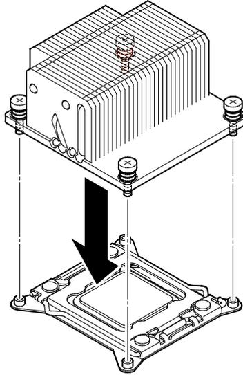
**Important** If you install additional CPU, ensure that the fins of the additional CPU's heat sink are in the same direction as those of the standard CPU.
