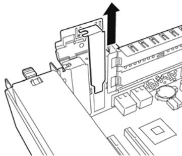
7. Install a PCI card in a PCI slot.
