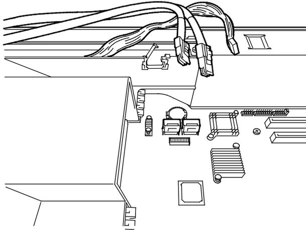
7. Remove the air duct.
