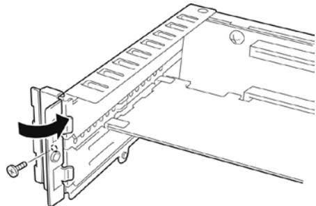
11. Install a Riser Card on the motherboard and secure it with three screws.
