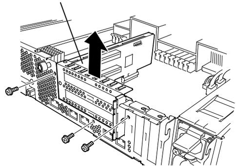
6. Remove one screw that secures the stopper and remove the stopper from the Riser Card.
