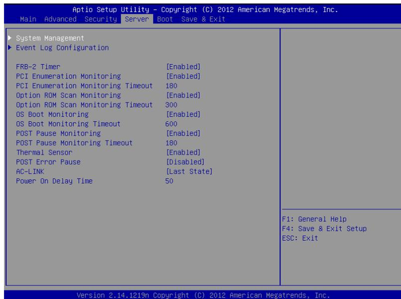
The **Server** menu screen shows the options you can configure and their features. For the menu **System Management**, move the cursor to it and then press **Enter** to show its submenus.
