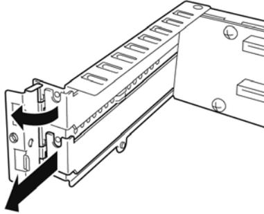
9. Install a PCI card in a PCI slot.
