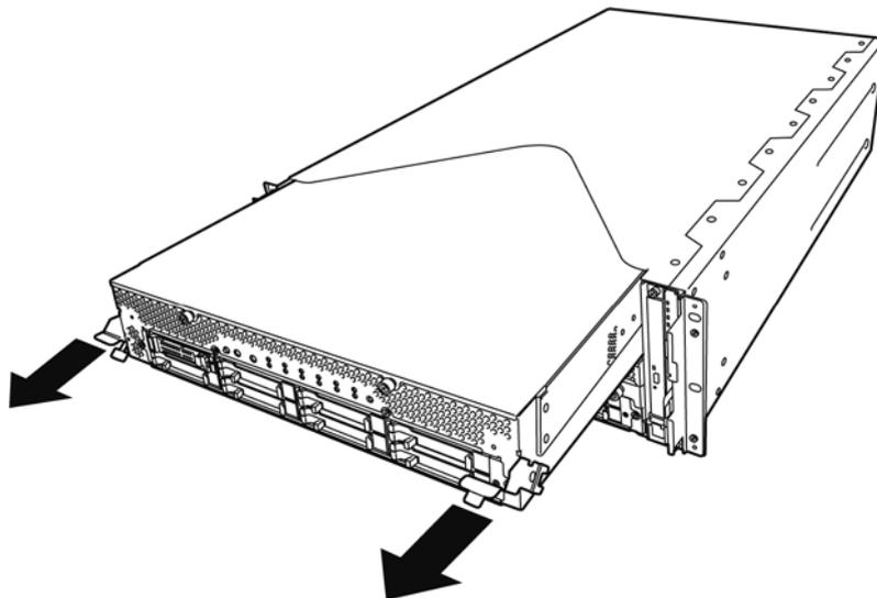
6. The CPU/IO module is locked on the way and cannot be pulled out. Lower the lock on the side of CPU/IO module to unlock it, and then pull it out.
