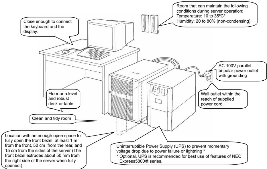
\* It is recommendable to use the server in a room where temperature can be kept between 15 and 25°C.
