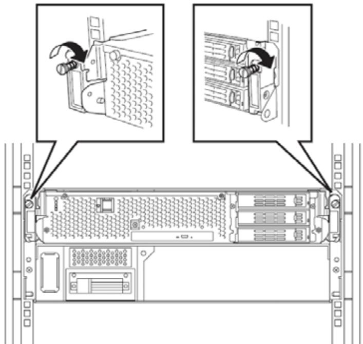
11. Mount the CPU/IO module 1 in the same way.
