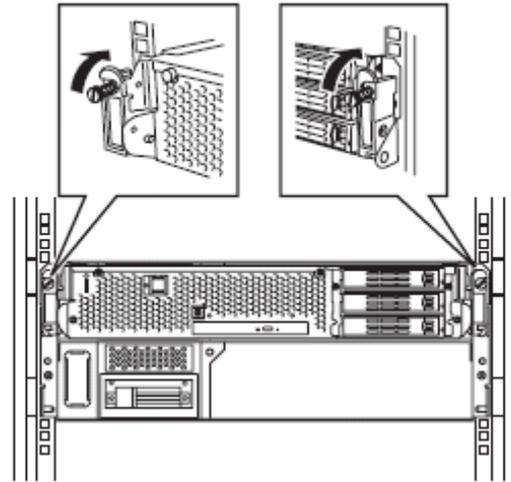
10. Fix the levers on the left and right sides by screws.
