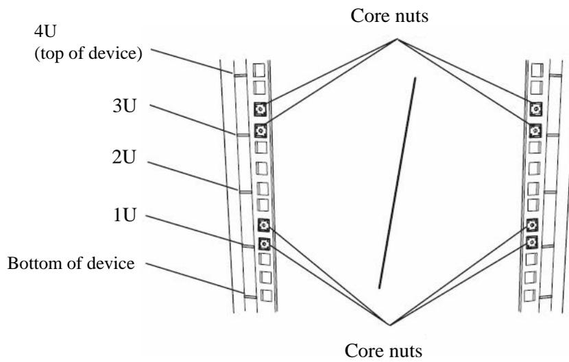
Fix a core nut from inside of the rack.
