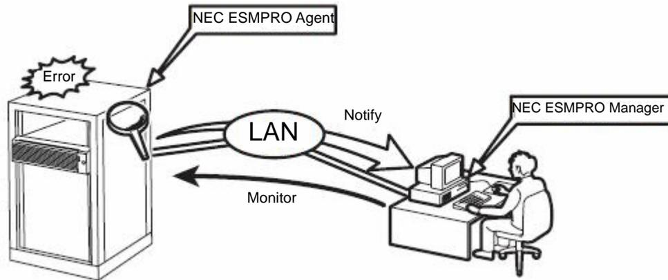
When a failing module in the server is to be replaced, NEC ESMPRO Manager enables logical module disconnection from the server and logical installation after module replacement.
