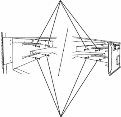
Washers for plate screw and plate screws (short)
