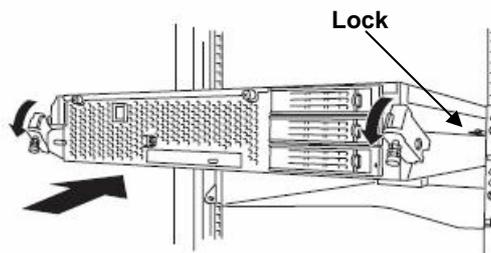
9. Lift the levers on the left and right sides to fix the CPU/IO module.
