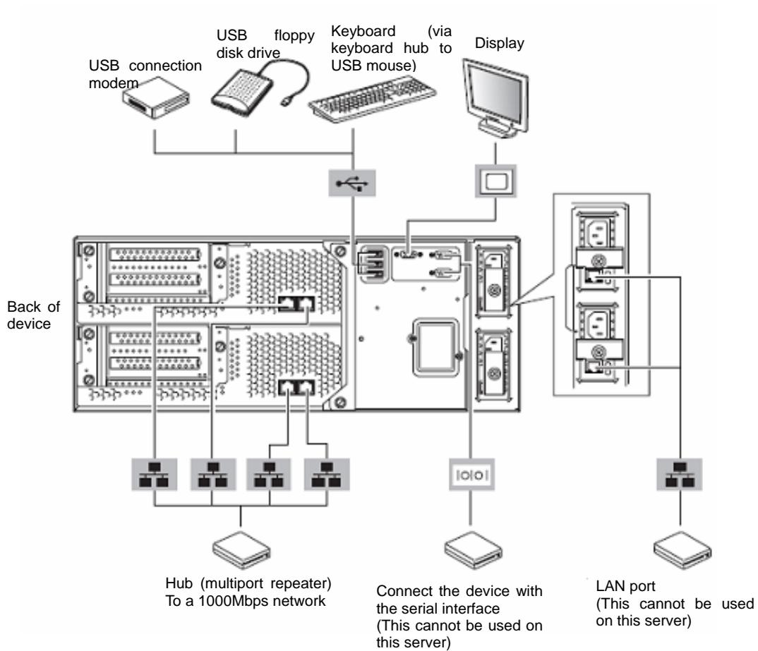
Rotate the stopper in clockwise direction, and insert the power cords to the AC inlets of the power unit.
