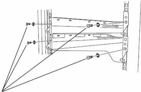
Washers for plate screw and plate screws (long)
