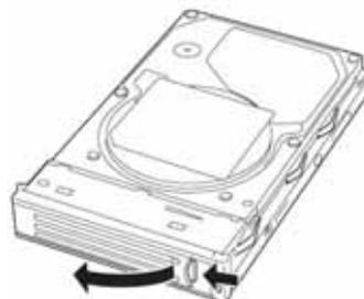
7. Firmly hold the handle of the hard disk to install and insert the hard disk into the slot.
