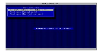
**IMPORTANT:** An initial selection of the menu is "Os installation". "Os installation" starts by the automatic after the Boot selection menu is displayed.
