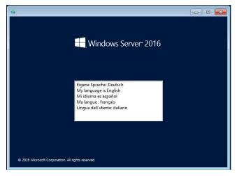
In case that "Windows Setup" window does not appear, <Enter> key was not pressed correctly in Step 2. Reboot the server and go back to Step 2. 4. Click Next.
