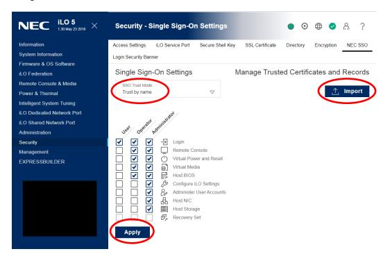
(6) Configure the value saved as "HOST\_NAME" in step (2) in text field of "Import Direct DNS Name" and click "Apply" button.
