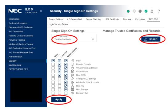
(14) Copy text of Certificate(\*1) generated in step (7) and paste it in text field. Then Click "Apply" button.
