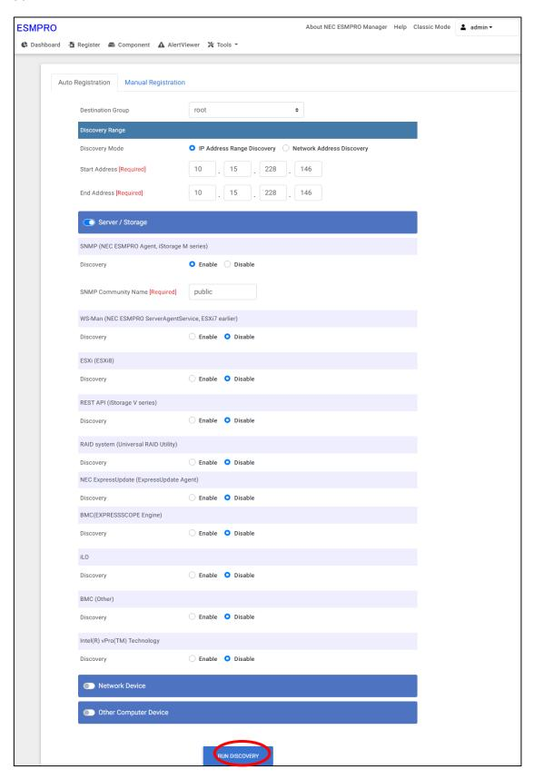
Click "RUN DISCOVERY" to discovery the managed components, and the "Auto Registration in Progress" screen will be displayed.
