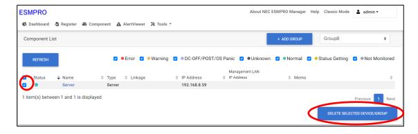
(3) Click "DELETE" and "Deleting components. Please wait a minutes." will be displayed. If the deletion finish, "The deletion process is complete." will be displayed, and click "OK".
