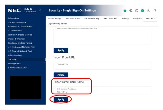
(7) Confirm if name set in step (6) is added in "Manage Trusted Certificates and Records" field on NEC SSO settings.
