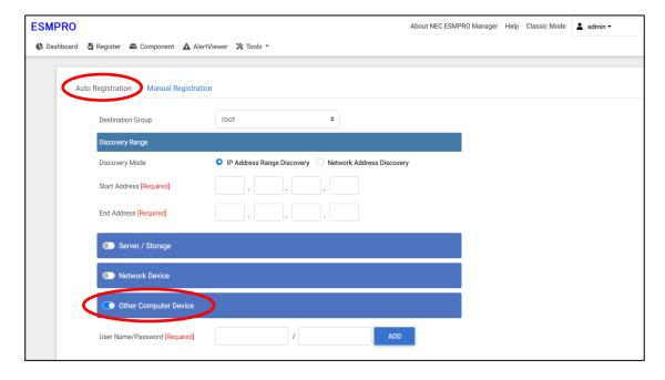
(3) Input the following items to search managed components based on Other Computer Device.
