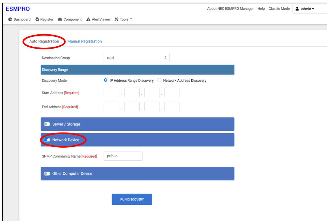
(3) Input the following items to search managed components based on Network Device.
