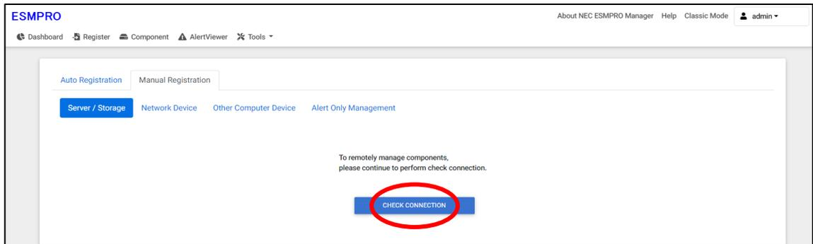
(6) If the "CHECK CONNECTION" is completed, “Connection check results” screen will be displayed.
