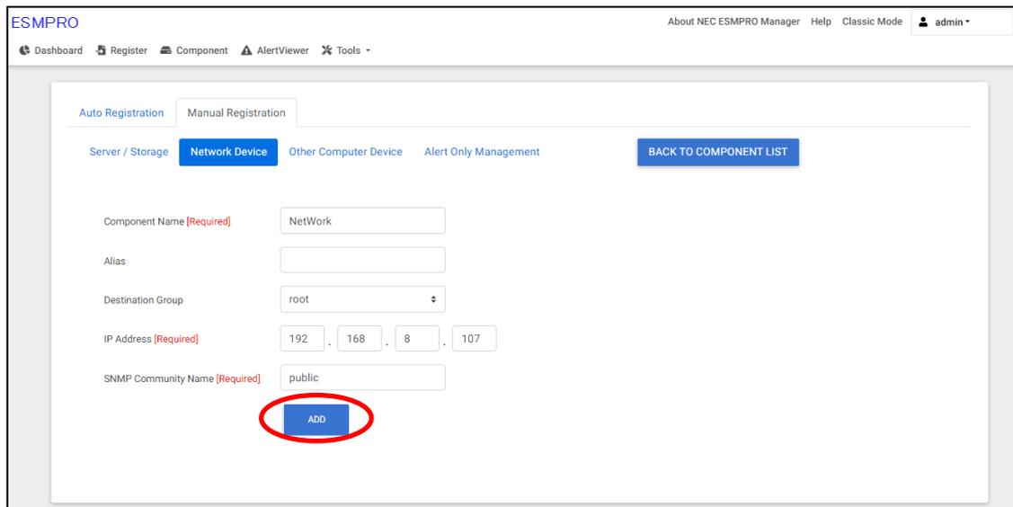
(5) The Network Device registered is displayed in "Component List"
