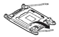
4. Raise the plate and set the Xeon processor to processor socket slowly.
