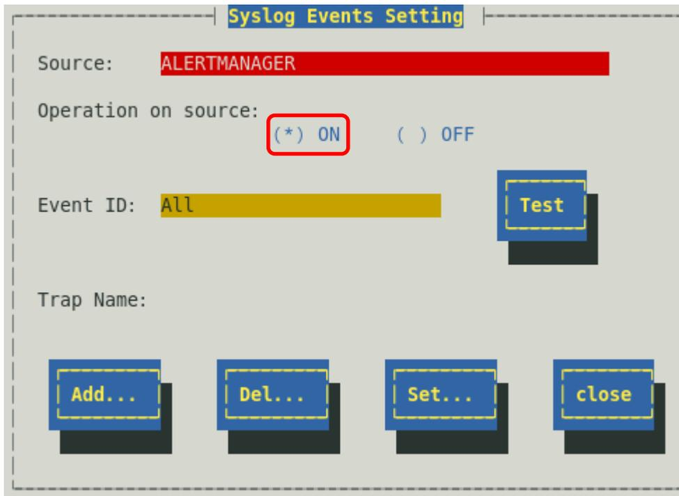
2. Select "ON" from "Operation on source". Set using <space> key.
