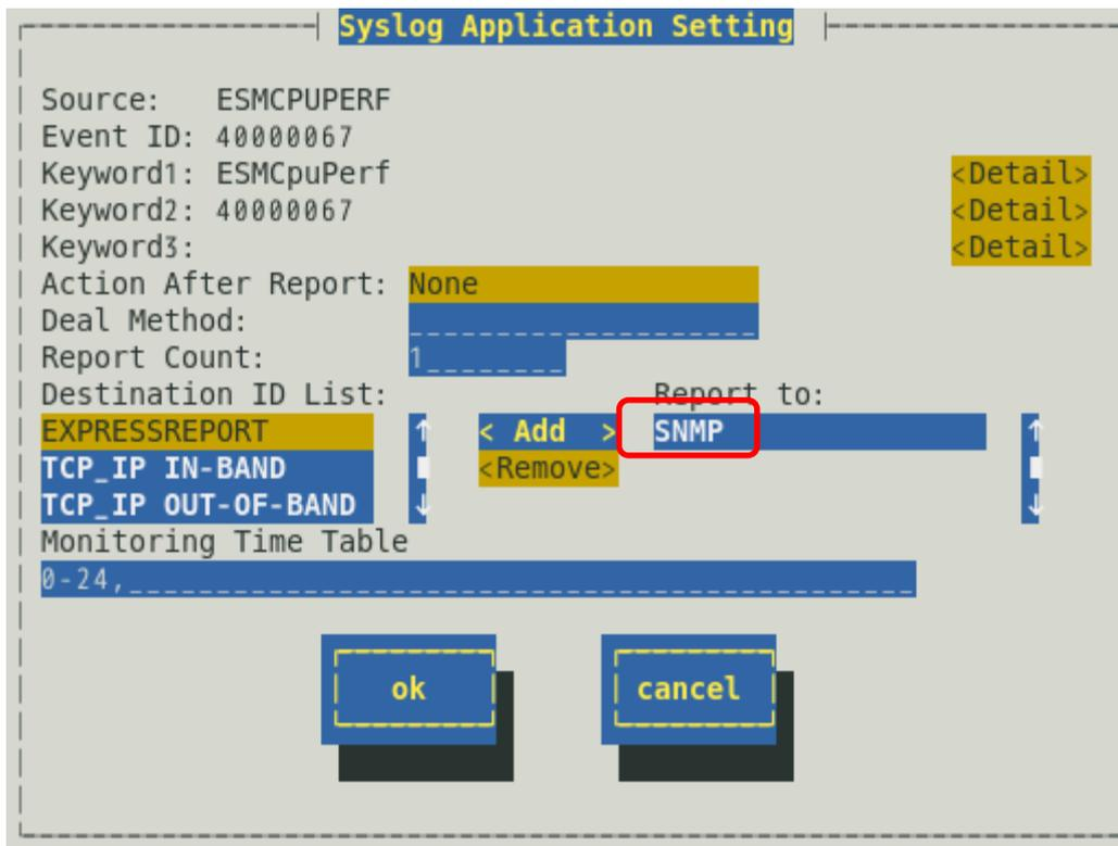
11. Select "SNMP" from "Report to" and press <Remove>. "SNMP" is deleted to "Report to".
