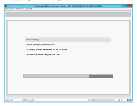
(3) Choose **Provisioning**. If no key is pressed within 10 seconds, the Provisioning will start automatically.
