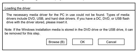
6. After connecting the removable media where the onboard RAID controller driver was copied, specify the path and click **OK**.
